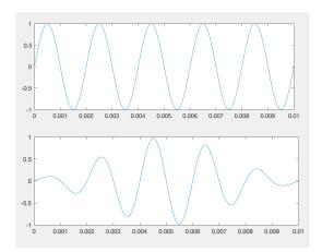
Using the same derived non-linear response technique described in the CEOAE simulation above, the OAE can be isolated from the stimulus. Tone bursts of 500, 1k, 1.5k, 2k, 3k, 4k, and 6kHz are simulated. Impulse responses and frequency responses are shown below.
