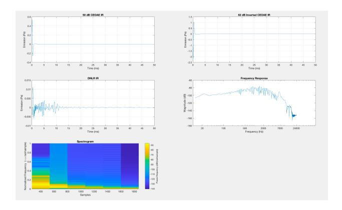
An FFT and spectrogram plot are also shown of the DNLR emission, without any time-windowing needed to remove the impulse. Because high frequency (basally located) OAEs will respond temporally sooner than low-frequency (apically located) OAEs, not needing to remove the early response with a time window will extend our OAE frequency response higher. We can see that our time-windowed CEOAE's frequency response does not show the notches above 7kHz that the DNLR's frequency response has.
